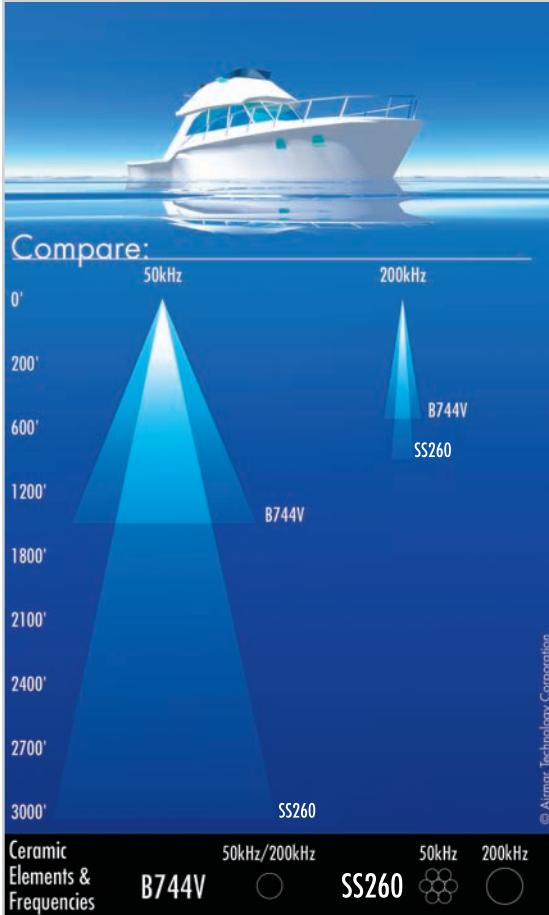
The image above shows the depth and beamwidth differences between the single-element, 600 W, B744V and the multiple-element, 1 kW, SS260.
