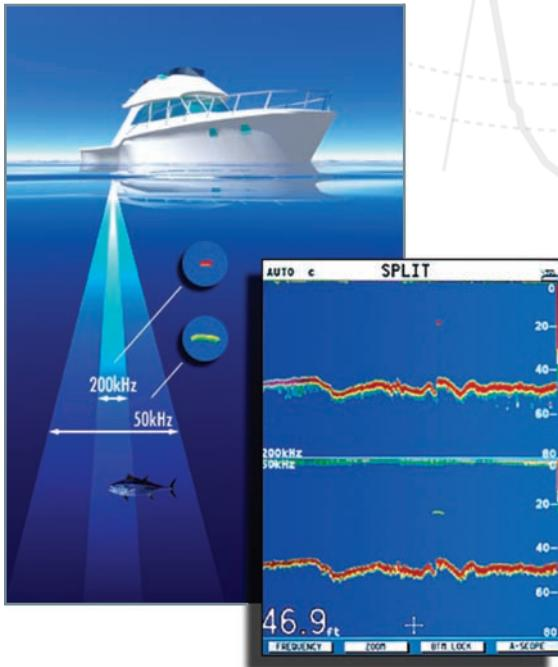
This illustration shows the differences in beamwidth of a transducer operating at both 50 kHz and 200 kHz. Notice the different way the fish appear as "marks" at each frequency.
